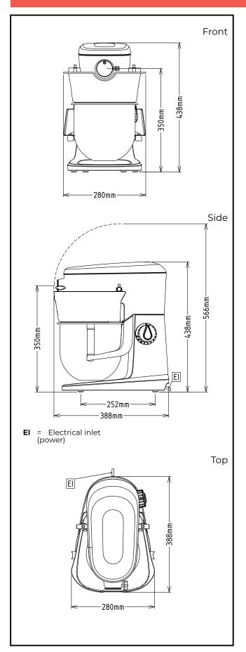
Electric Supply voltage: 603797 (DMX5BLCK) 200-240 V/1N ph/50/60 Hz **Total Watts:** 0.5 kW Capacity: Performance (up to): 0.75 kg/Cycle Capacity: 5.5 litres Key Information: External dimensions, Width: 280 mm External dimensions, 388 mm Depth: External dimensions, Height: 438 mm **Shipping weight:** 15 kg Net weight (kg): ISO 9001; ISO 14001 0.75 kg with Semi spiral **Cold water paste:** hook
